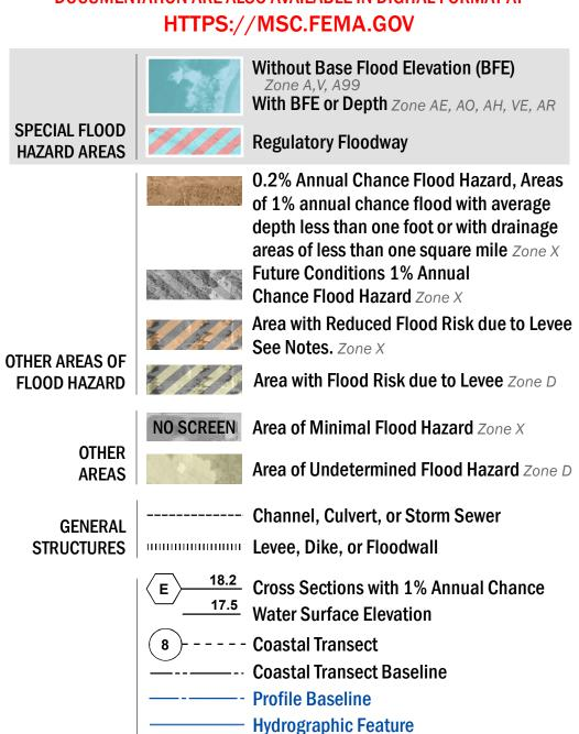
**Base Flood Elevation Line (BFE)**
