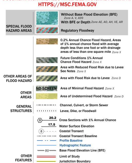
Note: Some Special Flood Hazard Areas with elevations may not appear with elevation labels if the Base Flood Elevation or Cross-section line which communicates the elevation for the location appears on the adjacent panel. Please see the Panel Locator Diagram on this map panel to determine the adjacent panel and find the elevation feature there, or alternatively use the Flood Insurance Study report for detailed elevations by flood source.
