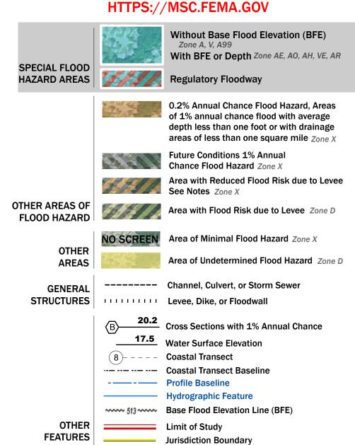
Note: Some Special Flood Hazard Areas with elevations may not appear with elevation labels if the Base Flood Elevation or Cross-section line which communicates the elevation for the location appears on the adjacent panel. Please see the Panel Locator Diagram on this map panel to determine the adjacent panel and find the elevation feature there, or alternatively use the Flood Insurance Study report for detailed elevations by flood source.
