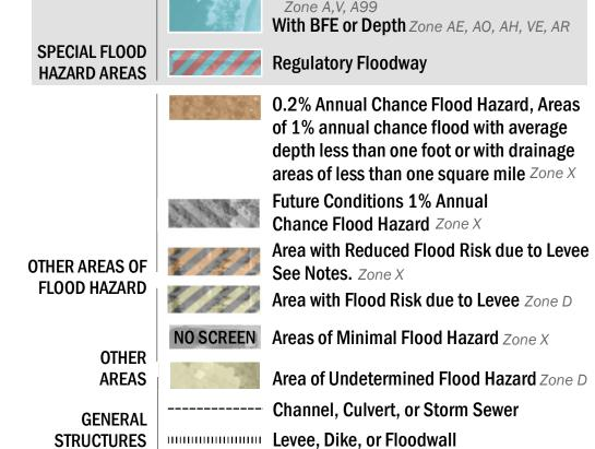
18.2 Cross Sections with 1% Annual Chance 17.5 Water Surface Elevation **Coastal Transect Coastal Transect Baseline** —- Profile Baseline Hydrographic Feature ----- 513 ---- Base Flood Elevation Line (BFE) Limit of Study OTHER
