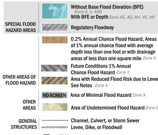
Area with Reduced Flood Risk due to Levee **Area of Undetermined Flood Hazard** *Zone D* 18.2 Cross Sections with 1% Annual Chance 17.5 Water Surface Elevation - - - Coastal Transect — -- Coastal Transect Baseline Profile Baseline **Hydrographic Feature** ----- 513 ---- Base Flood Elevation Line (BFE) Limit of Study OTHER **FEATURES Jurisdiction Boundary**
