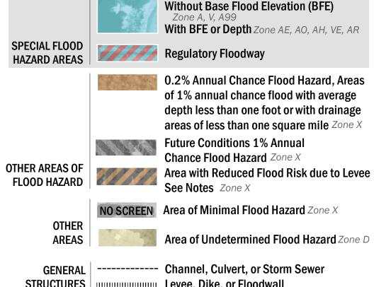
STRUCTURES Levee, Dike, or Floodwall 18.2 Cross Sections with 1% Annual Chance 17.5 Water Surface Elevation - - - - Coastal Transect — -- Coastal Transect Baseline - Profile Baseline - Hydrographic Feature ----- 513 ---- Base Flood Elevation Line (BFE)
