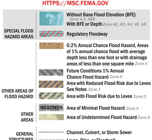
STRUCTURES Levee, Dike, or Floodwall 18.2 Cross Sections with 1% Annual Chance
