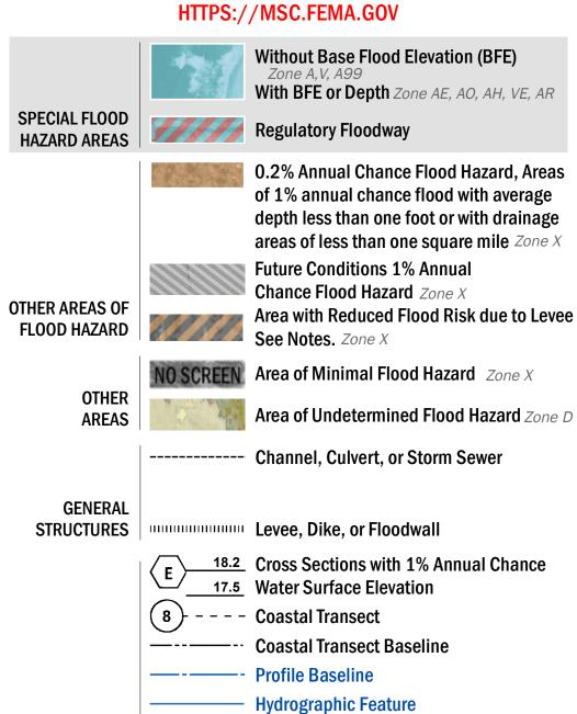
**Base Flood Elevation Line (BFE)**
